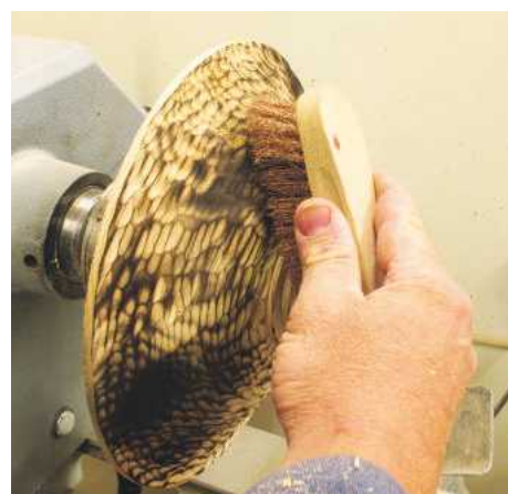
▲ Pic.15 You will need to remove the carbon before you put any finish onto the wood. A soft brass or a stiff bristle brush is best as anything too stiff like a steel brush would scratch the wood
